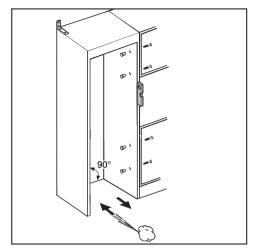
The housing unit must be carefully aligned using a spirit level before installing the appliance. The unit corners must be at right angles, as otherwise the furniture door will not align correctly with the 4 corners of the appliance.
